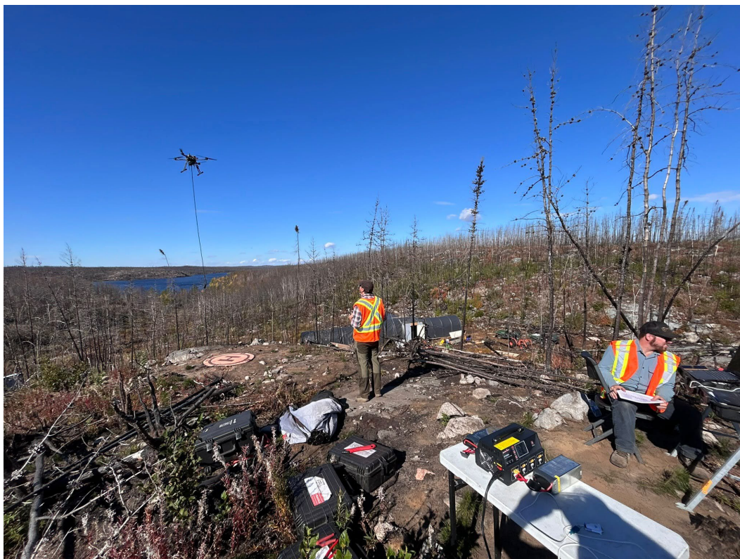
Figure 3: UAV magnetic survey in progress at the Munro Lake Project, September 2026.
